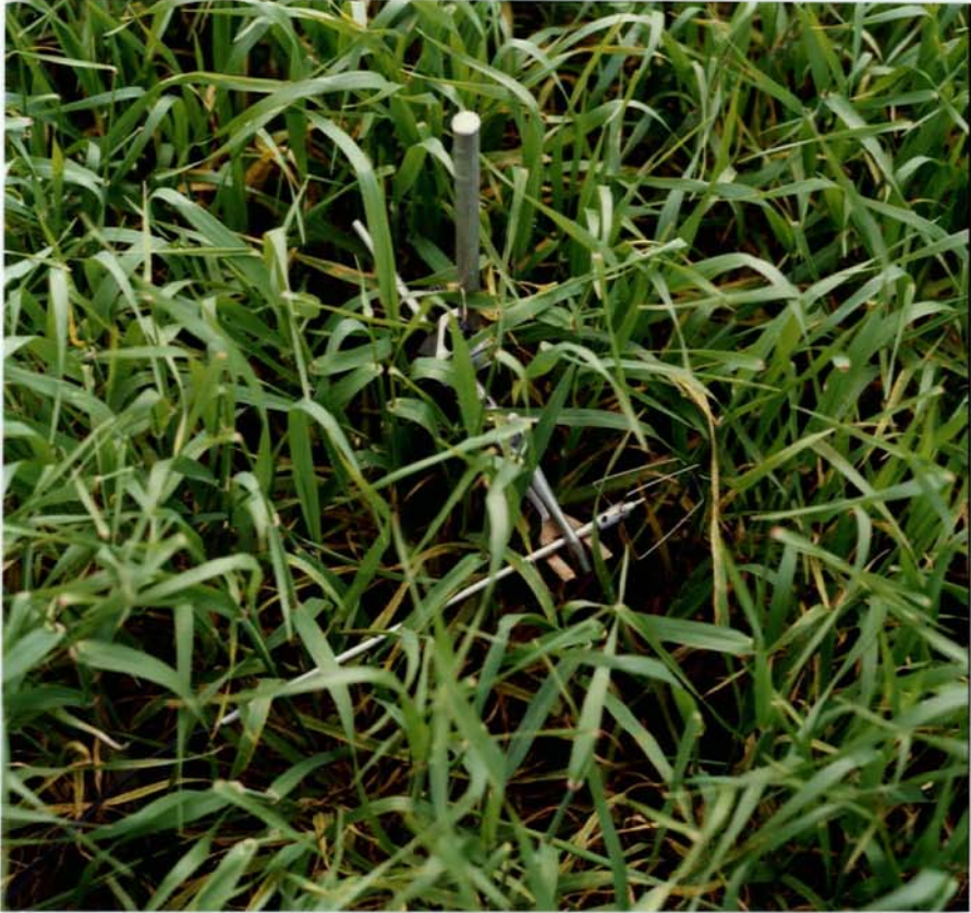
Figure 3 Mounting of triple-split film probe for measuring air flows within the crop canopy
